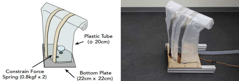
Figure 38: LiftTile actuator module.
